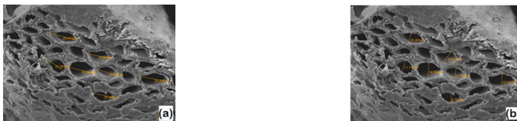
Figure.3. Scanning electronic microscopy ( with a magnification of 800x),(a) the opening of the pores on the x axis was marked (b)the opening of the pores on the y axis was marked
