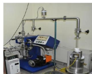
Figure.2. Sievert's apparatus setup for gaseous hydrogen charging
