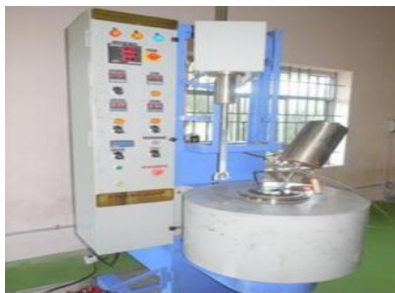
Figure 1. Experimental Setup of Stir Casting
