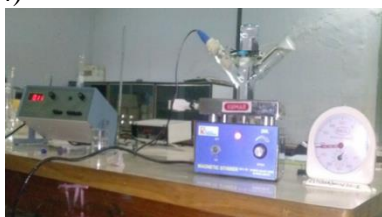
Figure.3. Actual set up for conductivity measurement in diffusion experiment and Franz cell also seen kept on magnetic stirrer, conductivity probe is also seen
