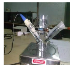
Figure.3. Actual set up for conductivity measurement in diffusion experiment and Franz cell also seen kept on magnetic stirrer, conductivity probe is also seen
