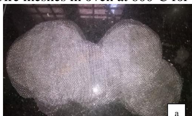
Figure.6. (a) Wire mesh substrate are cut in circular shape (b) Arranged calcined wire mesh substrate
