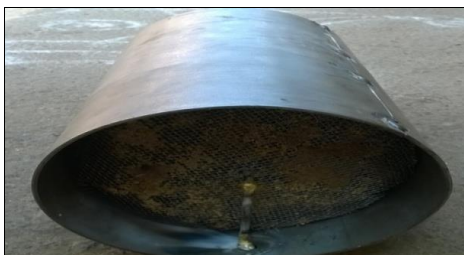
Figure.8. Coated wire mesh installed in outer shell of catalytic converter
