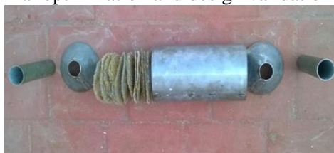
Figure.7. Collided view of catalytic converter
