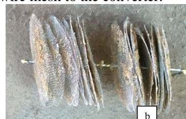
Figure.6. (a) Wire mesh substrate are cut in circular shape (b) Arranged calcined wire mesh substrate
