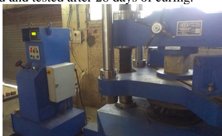
Figure.3.Testing of concrete cubes
