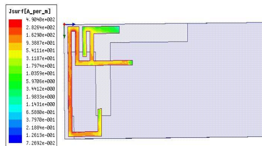
Figure.12. Current distribution in the proposed antenna.
