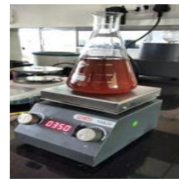
Figure.3. Stages of Enzymatic transesterification process: (A) Xylanase lipase; (B) Weighing of lipase; (C) Blending of BAO and methanol in conical flask as per molar ratio; (D) Conical flask mounted on magnetic stirrer at constant stirring speed of 350 rpm
