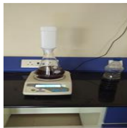
Figure.3. Stages of Enzymatic transesterification process: (A) Xylanase lipase; (B) Weighing of lipase; (C) Blending of BAO and methanol in conical flask as per molar ratio; (D) Conical flask mounted on magnetic stirrer at constant stirring speed of 350 rpm
