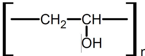
Figure.5. Molecular Structure of Poly Vinyl Alcohol (The value of 'n' lies between 500 to 5000)
