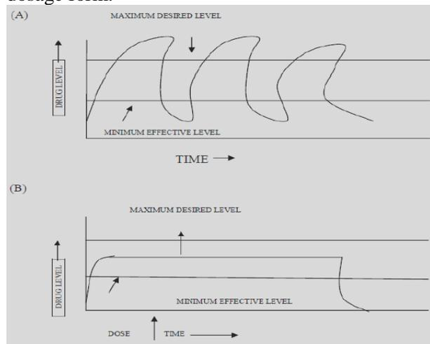
**Figure.1. Showing the difference between conventional drug delivery system and sustained release drug delivery system.**
