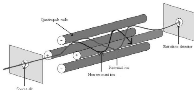
Figure.6. Schematic of the Triple Quadrupole Mass Spectrometer
