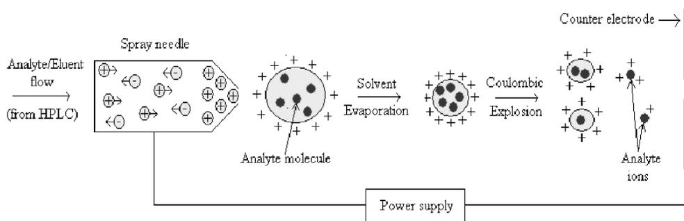
Figure 4. Adapted schematic of electrospray ionisation
