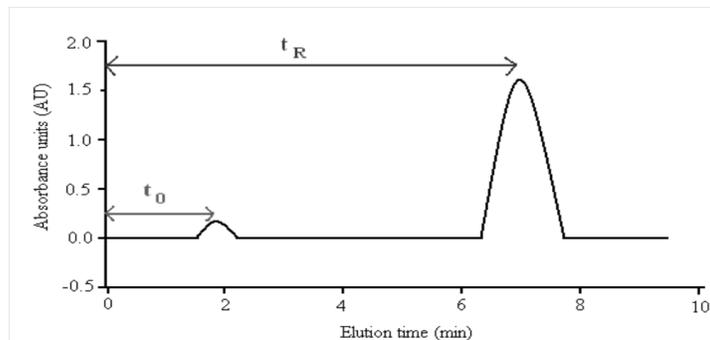
**Figure.1.Schematic of a typical HPLC chromatogram**
