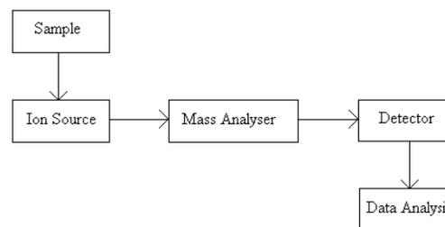
Figure 3. A schematic of the principle components of a MS
