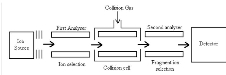
**Figure no 5: Adapted schematic of a Quadrupole Mass Analyser**
