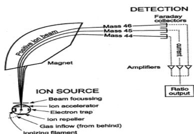
Figure 2. Schematics of a simple mass spectrometer with sector type mass analyzer
