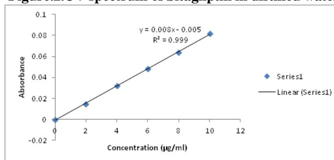
Figure.3.Calibration curve of SITA by UV method
