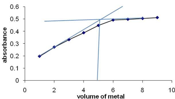
**Figure.6.Mole ratio method for CP complex with Hg(II) ion at 420nm**
