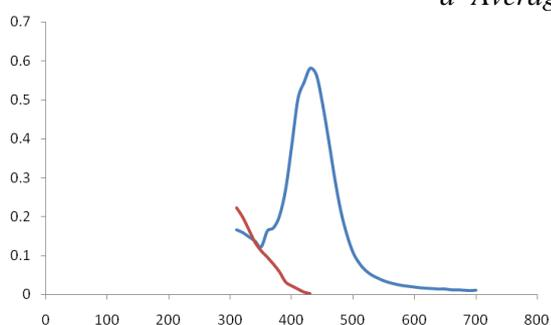
**Figure.2.Absorption spectra of 55.7 $\mu\text{g/ml}$  CP complex with  $1 \times 10^{-2}\text{M}$  Hg(II)**
