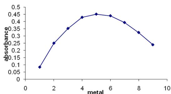
**Figure.5.Job's method for CP complex with Hg(II) ion at 420nm**
