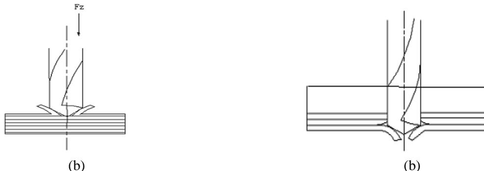
**Fig.1. Drilling induced damage, (a) Peel-up, (b) Push-down delamination <sup>(26)</sup>**
