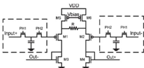
Fig.3.Input sample/hold and Voltage to Current converter
