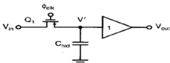
Fig. 1 Open loop sample and hold circuit
