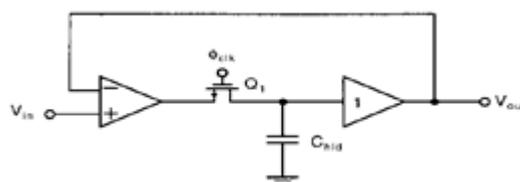
Fig. 2 Closed loop sample and hold circuit
