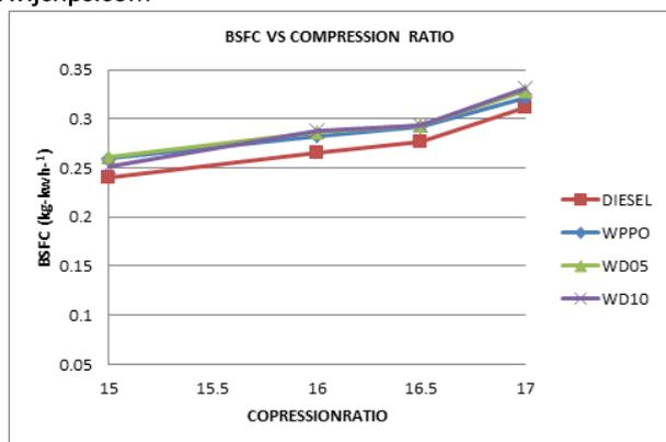
Figure 4. Brake Specific Fuel Consumption vs. Compression ratio
