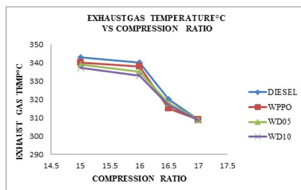
**Figure.3.Exhaust gas temperatures vs. Compression ratio**
