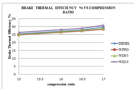
**Figure.2.Brake Thermal Efficiency vs. Compression ratio**
