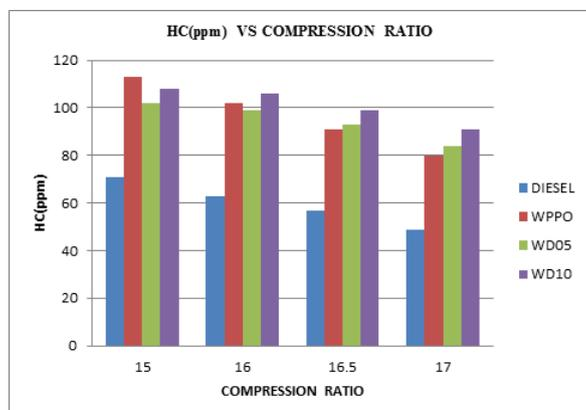
Figure 8. HC Emissions vs. Compression ratio
