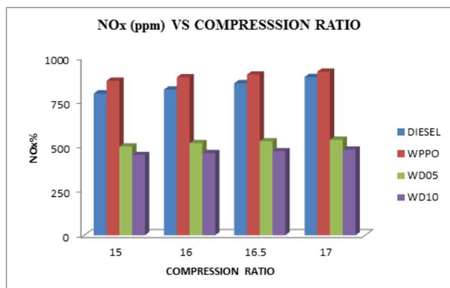
Figure 6. NO<sub>x</sub> Emissions vs. Compression ratio
