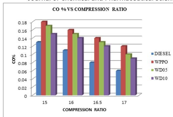
Figure 5. CO Emissions vs. Compression ratio
