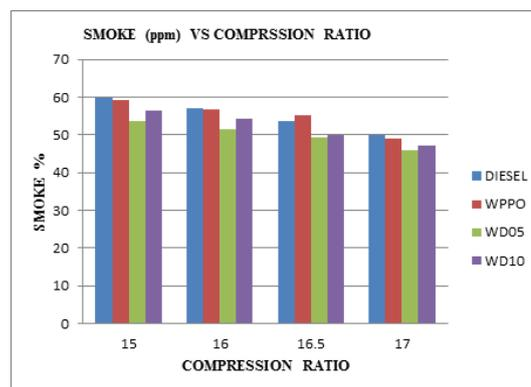
Figure 7. Smoke Opacity vs. Compression ratio
