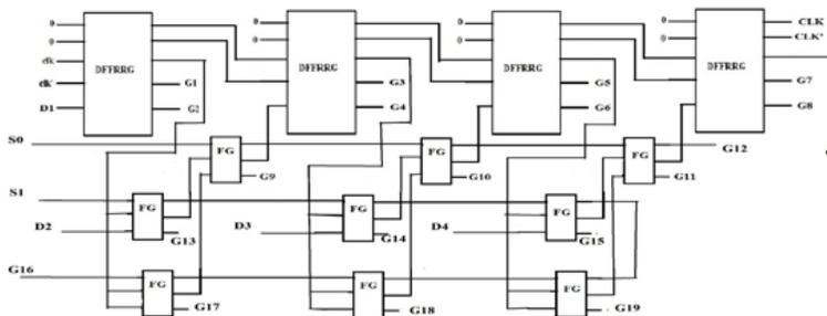
**Fig.1. Reconfigurable shift register architecture using RR- Fault Tolerant Reversible Logic Gate.**
