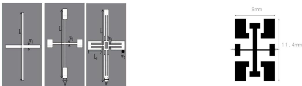
Figure 1. Geometries of 4 types of DGS : (a) Cross (b) Dumbbell (c) E-shape (d) Proposed shape
