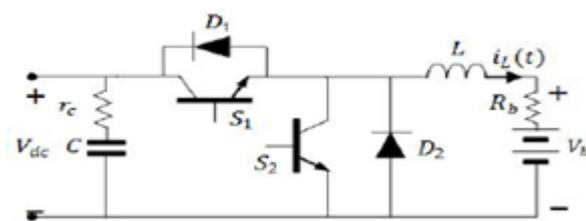
**Fig. 3. A buck converter with two-quadrant switches and bidirectional power flow.**
