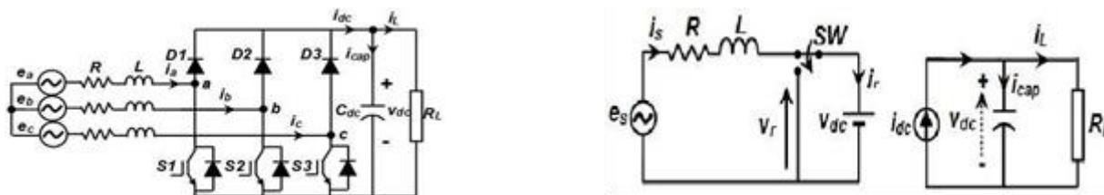
**Fig. 1. Ac-dc PWM semi-controlled rectifier. (a) Power circuit, (b) per-phase input equivalent circuit, (c) output equivalent circuit**
