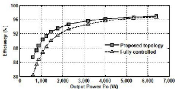
**Fig. 4. Estimated efficiencies for the proposed topology ( $\eta_1$ ) & the fullycontrolled topology ( $\eta_2$ )**
