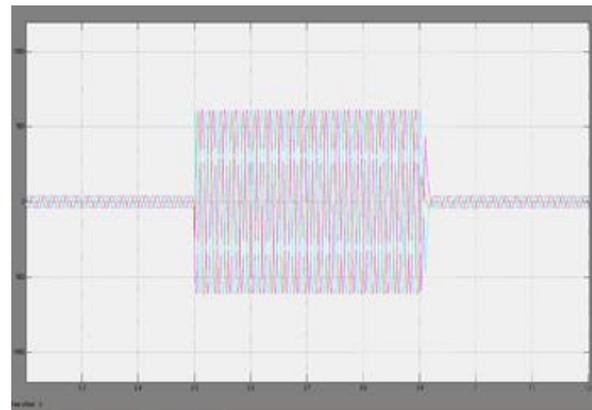
**Fig.4.Injected voltage for sag compensation**
