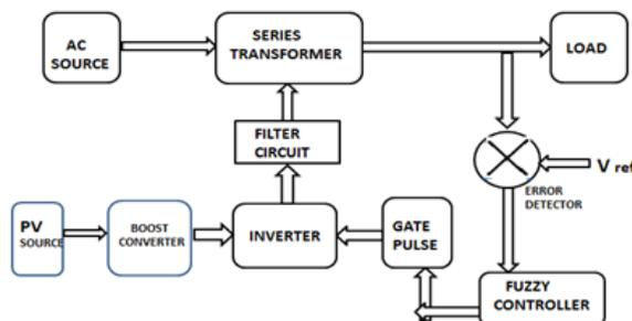
**Fig.1. Proposed System Block Diagram**
