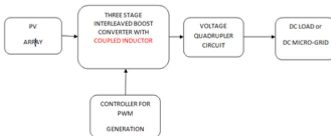
The output of the voltage quadrupler circuit is connected into a DC load or DC micro Grid. The work of voltage quadrupler is increasing four times of the voltages.
