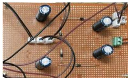
Fig.1.2.Voltage Quadrupler Hardware
