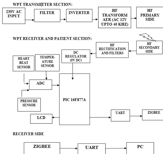
**Fig.1. Block Diagram of Wireless Power Transmission**
