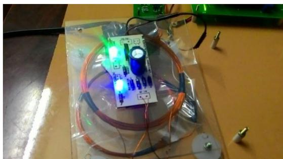
**Fig.6. Transmitter Section of the Circuit**
