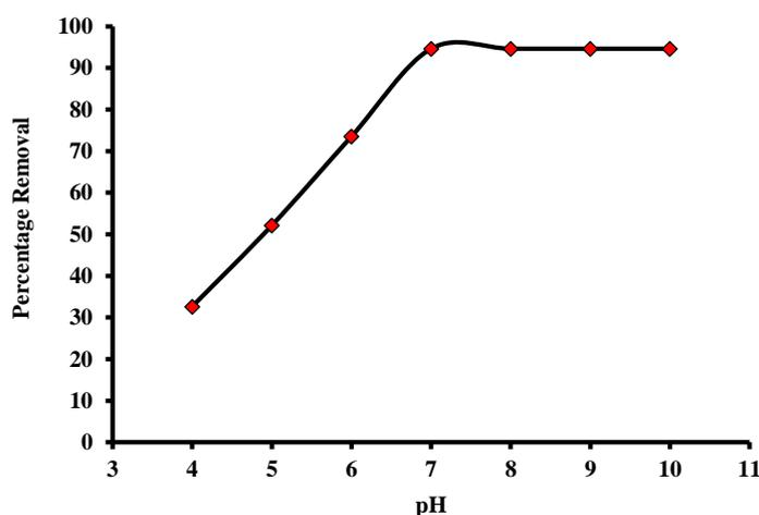
Fig.5. The percentage reduction of color in a textile industry wastewater using *Lemna minuta L.* against pH
