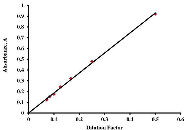
Fig.2. Calibration curve for textile industry wastewater at a wave length of 506 nm
