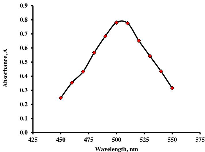
Fig.1. Absorbance curve for textile industry wastewater
