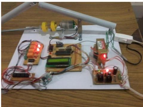
**Fig.4.A prototype of automatic physiotherapy machine**
