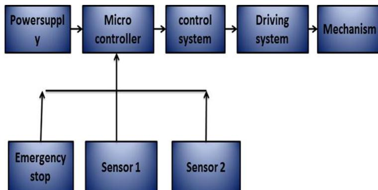
**Fig.3. Block diagram of automatic physiotherapy machine**
