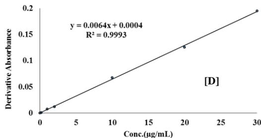
**Figure. 6. Calibration curves of Brimonidine tartrate**
