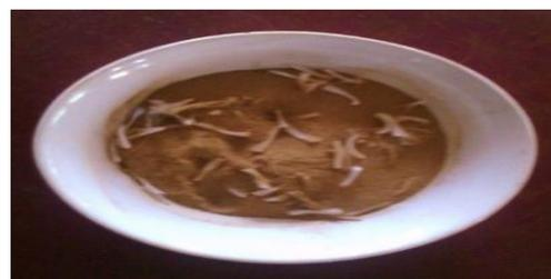
Fig.5.Soil Specimen Randomly Mixed with Fibers
