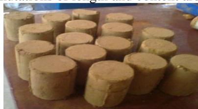
Fig.7. Fiber reinforced soil specimen
