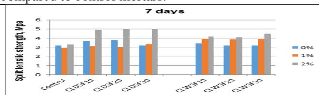
**Fig. 6 Split tensile strength of mortars with silica fume/basalt fiber (0, 1 and 2%) for 7 days of curing**
