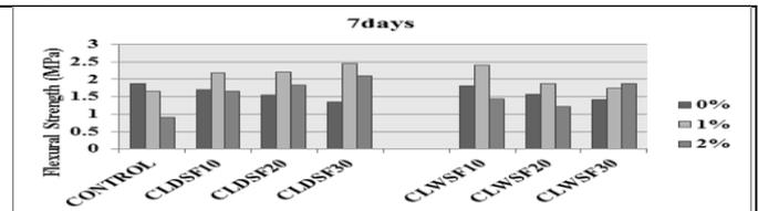
**Fig.8.Flexural Strength of mortars with Silica Fume/Basalt Fiber (0, 1 & 2%) For 7 Days of Curing**
