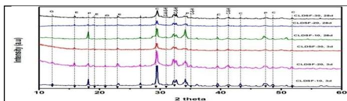
**Fig.3.** XRD of different mixes LD series with SF at 3 and 28 days
