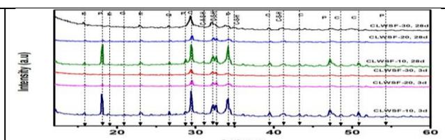
**Fig.4.** XRD of different mixes LW series with SF at 3 and 28 days
