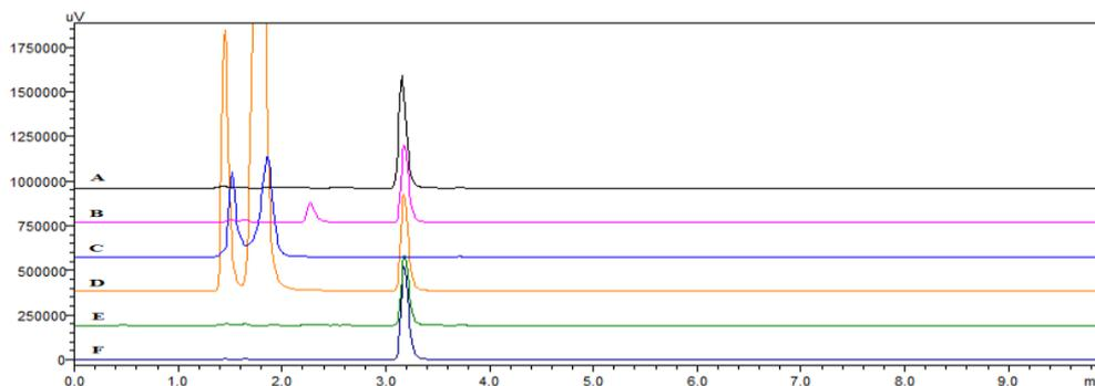
**Figure.3. Typical chromatograms of Cabazitaxel (100 µg/ml) [A], acidic [B], alkaline [C], oxidative [D], thermal [E], and photolytic [F] degradations**
