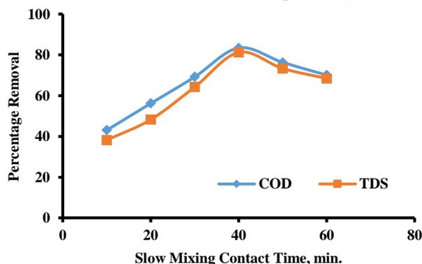
**Fig. 2 Effect of slow mixing contact time by orange peel activated carbon powder**
