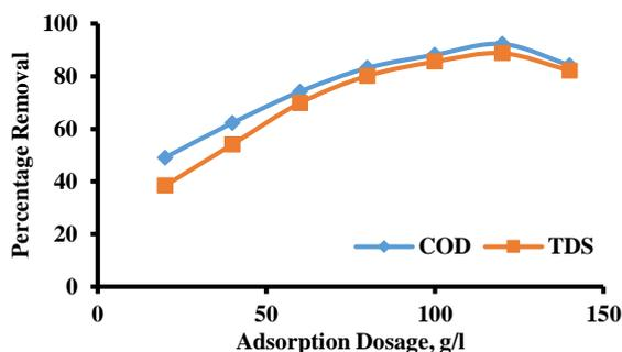
**Fig. 3 Effect of adsorbent dosage by orange peel activated carbon powder**
