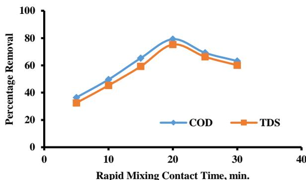
**Fig. 1 Effect of rapid mixing contact time by orange peel activated carbon powder**
