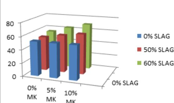
**Figure 10 Comparative Study on Compression strength with respect to replacement of Slag**
