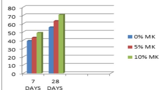
**Figure 7 Comparative Study on Compression strength with respect to replacement of Metalaolin**
