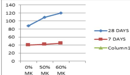
**Figure 8 Comparative Study on Compression strength with respect to replacement of Metalaolin**
