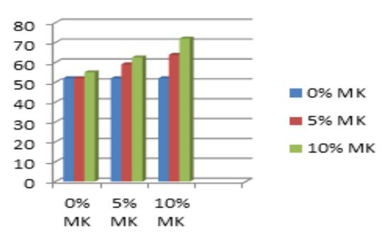
**Figure 9 Comparative Study on Compression strength with respect to replacement of Metalaolin**
