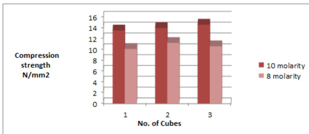
**Figure 3. Chart of Compressive Strength for Curing of Geopolymer Concrete Cubes for 28 Days**
