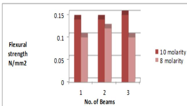
**Figure 1. Chart of Flexural Strength of Geo polymer Concrete Beam for 28 Days**
