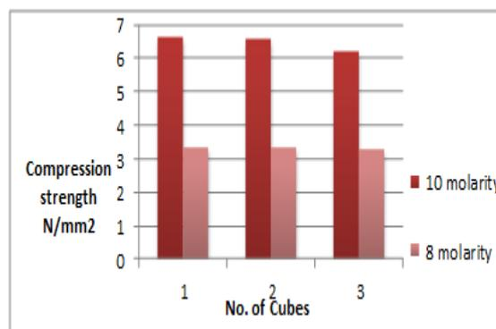
**Figure 2. Chart of Compressive Strength for Acid Resistant Test of Geo polymer Concrete Cubes for 28 Days**
