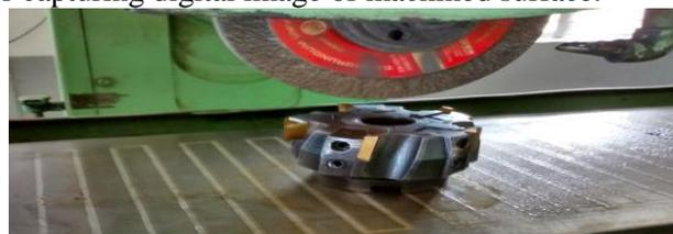
Fig.4. Fault creation using surface grinding machine
