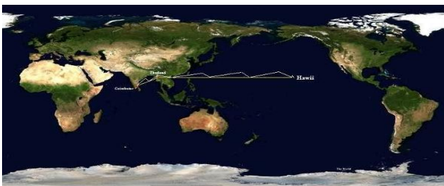
Figure.6.Number of Hops that Signal Experienced on its way to the receiver from NPM Transmitter
