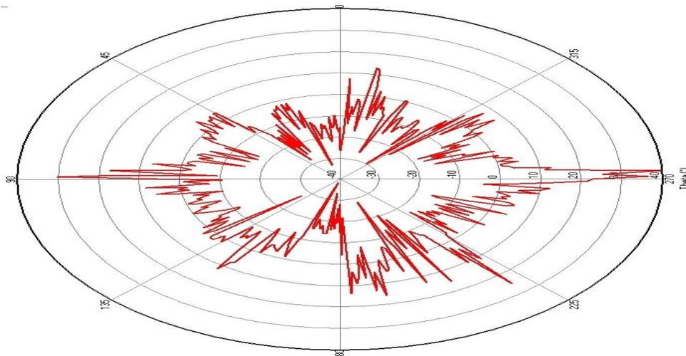
**Fig. 5. RCS Scattering plot for 12 wind turbines**
