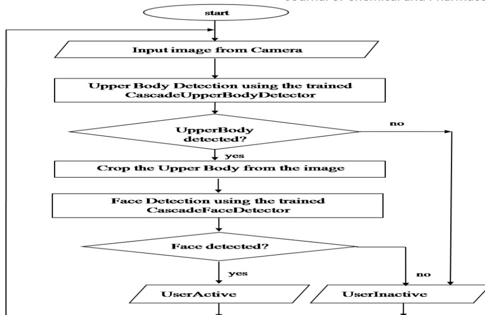
**Figure.2. The flow chart of the User State Recognition module**
