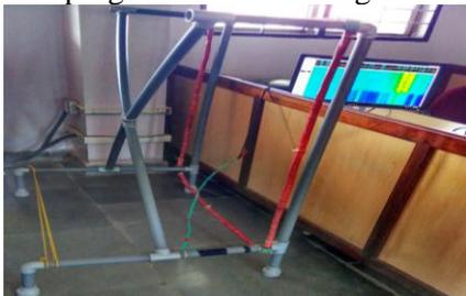
**Figure.1. The VLF loop antenna and system running the spectrum lab software**
