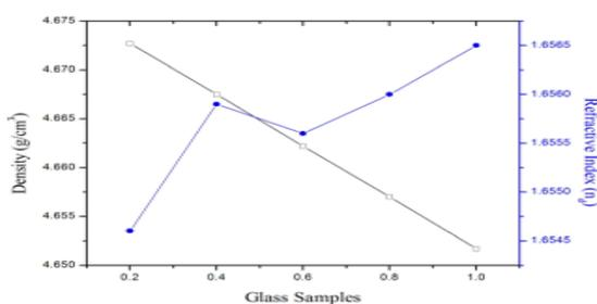
**Fig.1. Variation of density and refractive index as a function of  $\text{CaO-PbO-B}_2\text{O}_3\text{-SiO}_2\text{: Pr}_2\text{O}_3$  glasses**
