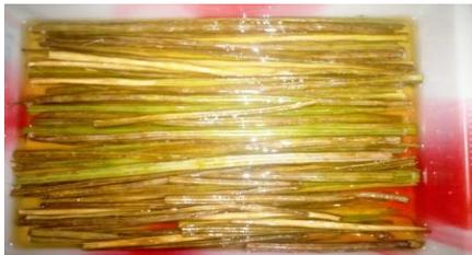
Figure.2. Fibres Treated in NaOH and Fibres in Dry Condition
