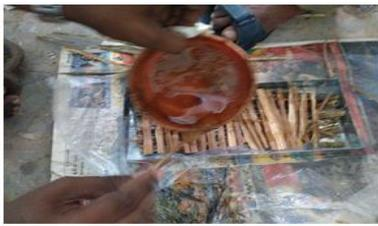
Figure.3. (a) Alignment of Fibre and (b) Resin is applied
