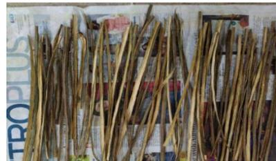
**Preparation of composites:** The composite has been with three layers of drumstick fiber. The polyester resin mixture was poured into mould plate, then drumstick fiber was placed in the mould plate (hand layup) and then polyester resin mixture was applied. After that weight has been applied manually around 25 kg and then it has been kept for 24 hours for curing.
