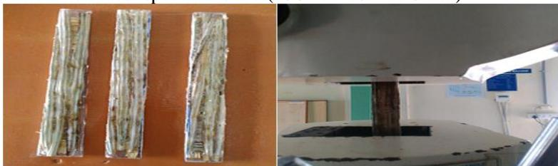
Figure.5. Tensile test specimens (a).before test, (b)Tensile piece loaded for tensile testing(250mm\*25mm\*5mm)
