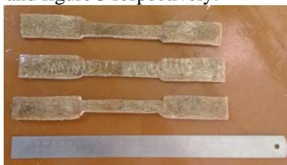
Figure.4. Specimen for tensile test
