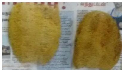
Figure.3. Fiber after NaOH treatment
