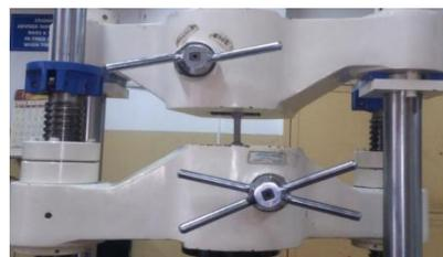
Figure.5. Loading arrangement of specimen
