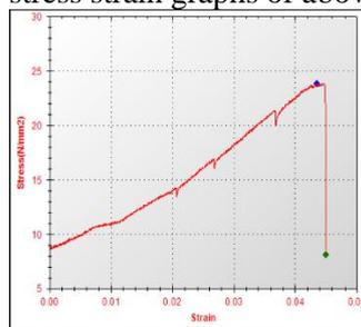
**Figure. 10(b). Stress vs strain graph of HCl treated Sugarcane fiber composite**
