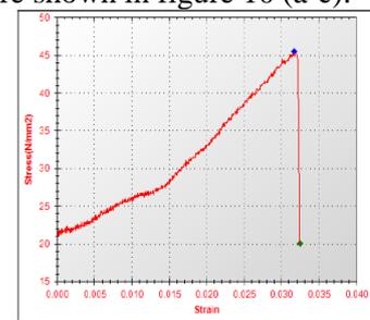
**Figure. 10(c). Stress vs strain graph of NaOH treated Sugarcane fiber composite**
