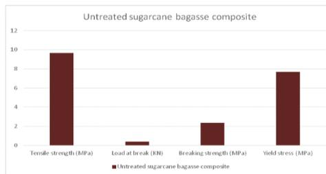
Figure.7. Tensile properties of untreated sugarcane bagasse composite
