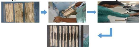
Figure.4. Flow chart for specimen preparation
