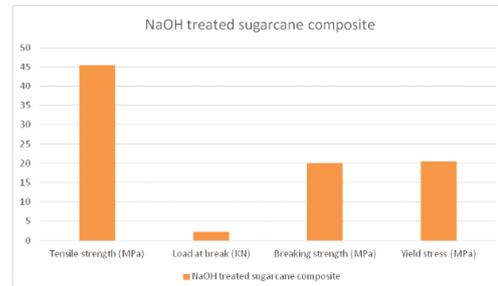
**Figure.9. Tensile properties of NaOH treated sugarcane bagasse composite**
