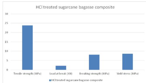
**Figure.8. Tensile properties of HCl treated sugarcane bagasse composite**
