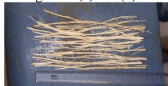
Figure. 1(b). Prepared Sugarcane fiber
