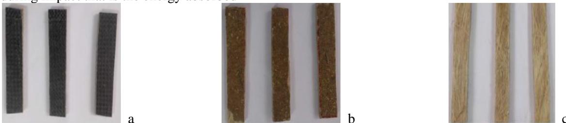
**Fig.3. Tested specimen of before tensile test (a) carbon, sisal and rice husk (b) sisal and rice husk (c) sisal, banana and kenaf**
