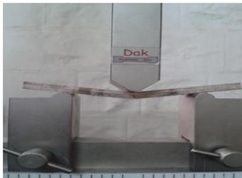
**Fig.2. Flexural testing**
