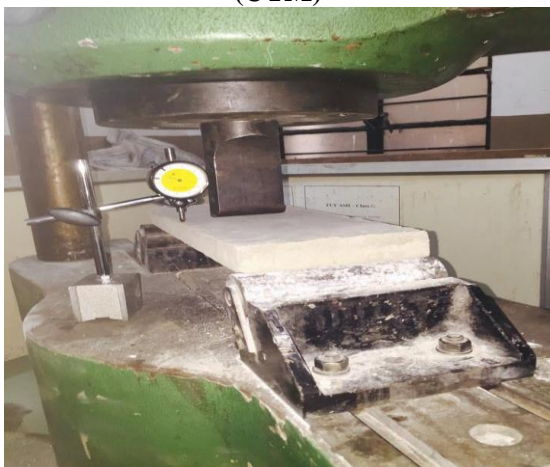
Figure.3. Deflectometer placed over the slab
