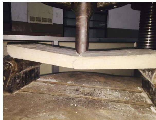
Figure.4. Crack in progress in slab
