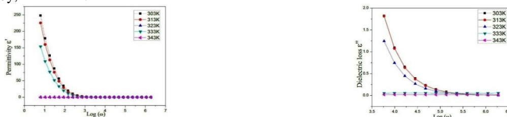
Fig.2. Dielectric constant ( \epsilon' ) and dielectric loss ( \epsilon'' ) versus \log(\omega) for PEO/PVA doped with 10 wt% of \text{NH}_4\text{Cl} at different temperatures
