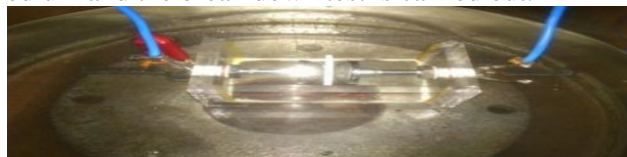
Figure.3b.Electrode Setup for the measurement of AC Breakdown Voltage
