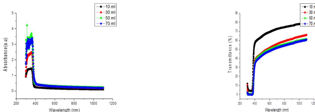
Figure.3(a)absorbance and (b) transmission spectra of various solution quantity of ZnO thin film
