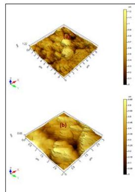
Fig.2. AFM images of (a) 30 ml (b) 70ml of ZnO thin film
