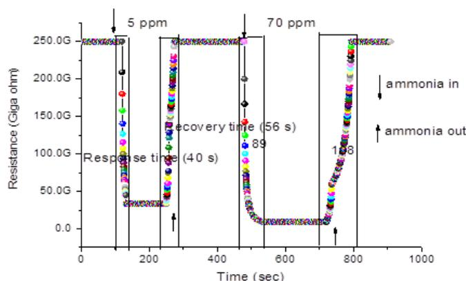
**Fig.4. Resistance response of 5 and 70 ppm at room temperature**
