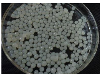
Fig.1. Chitosan beads prepared by a new method without a cross linking agent
