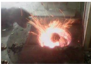
Fig. 2 Addition of activated carbon particles in to the molten metal
