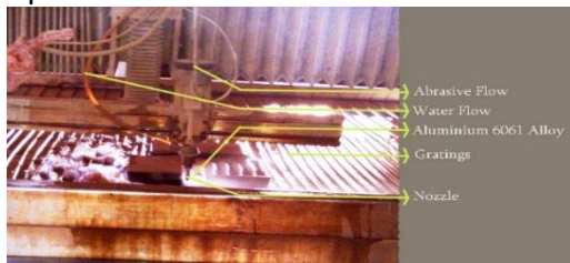
Fig.3.Experimental Setup of AWJM with Mixing Chamber
