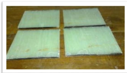
Fig.2. GFRP Laminate [0] Orientation – unidirectional ply
