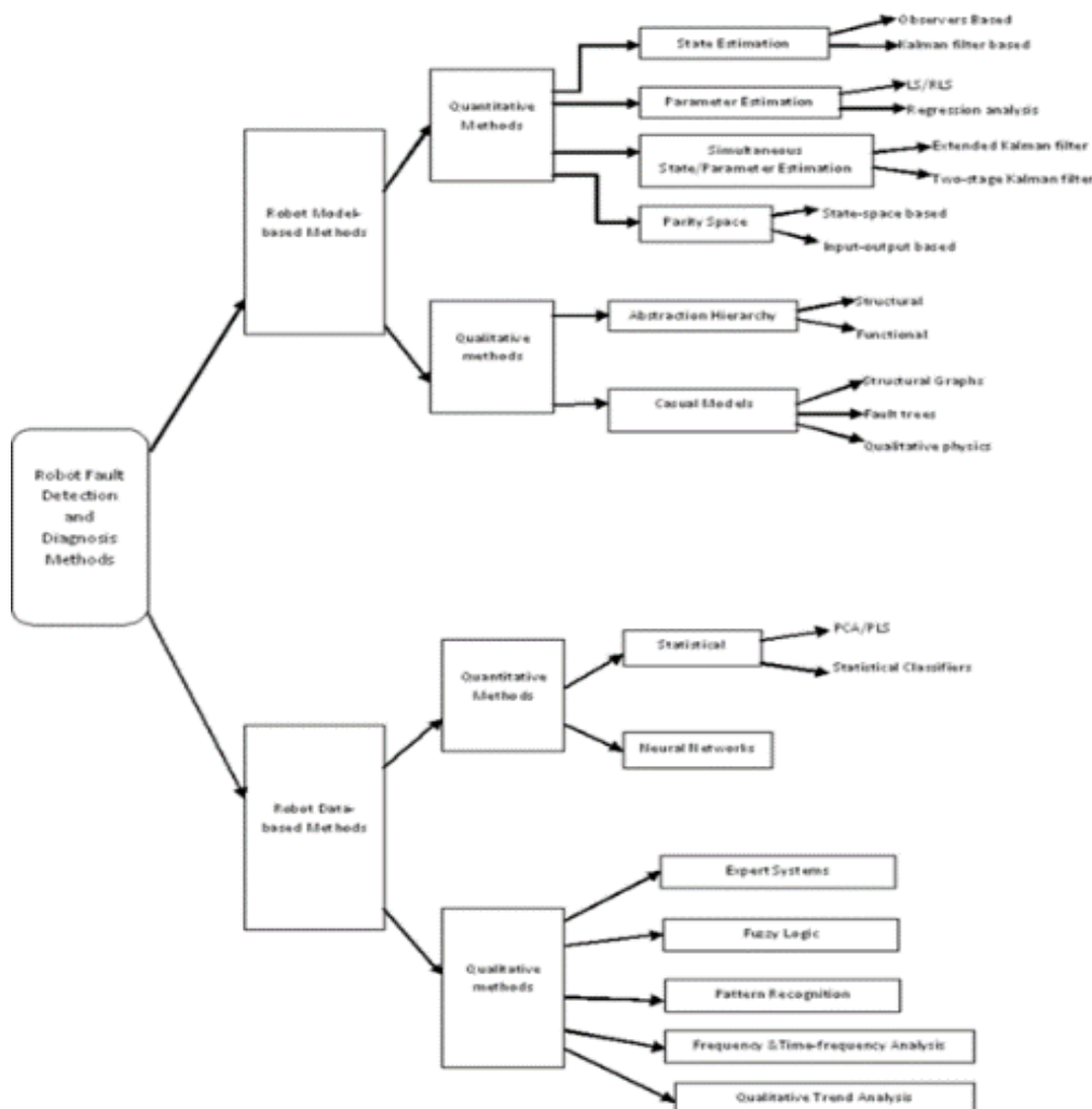
Fig.4. Robot fault detection and diagnosis algorithms
