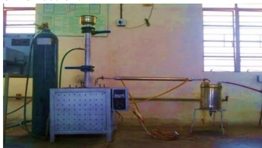
Fig.1. Pyrolysis reactor experimental set up
