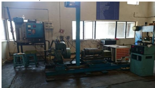
Fig.2. Photographic view of Engine test set-up.
